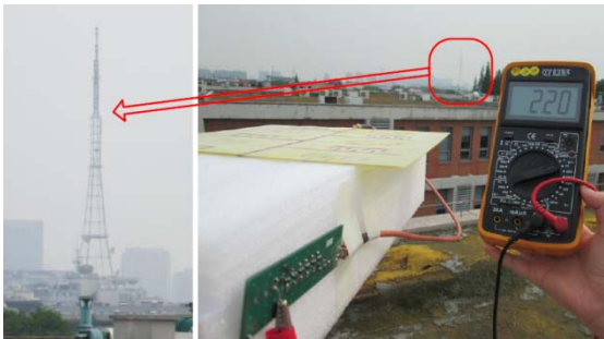
Fig. 6. Field measurement in downtown Suzhou, China, with the test prototype system harvesting wireless energy from digital TV signals broadcasted from Suzhou TV tower.
